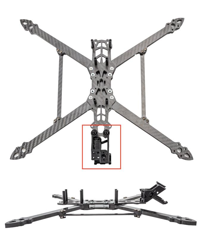
Fasten the print to the middle board as shown in the diagram
